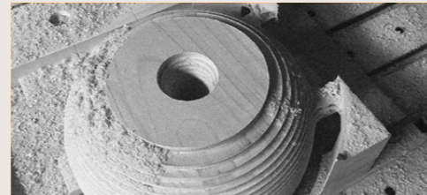
2. CNC roughing pass to set proportions
